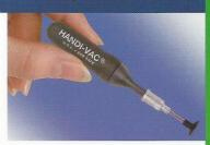
Our vacuum-bulb type tools are the lowest cost pick-and-place tools available. These tools operate very similar to a tweezer. Simply squeeze the vacuum bulb, place the soft suction cup to the part to be handled, then relax your squeeze and the part is firmly gripped. A second squeeze releases the part.
